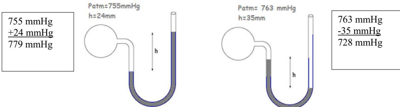
***Open manometer. Look at whether the liquid in the tube is higher on the side of the container or the open end of the tube. If it is closer to the open end, you add the atmospheric pressure to the height difference of the liquid in the tube. If it is closer to the container, you subtract the atmospheric pressure to the height difference of the liquid in the tube.***
